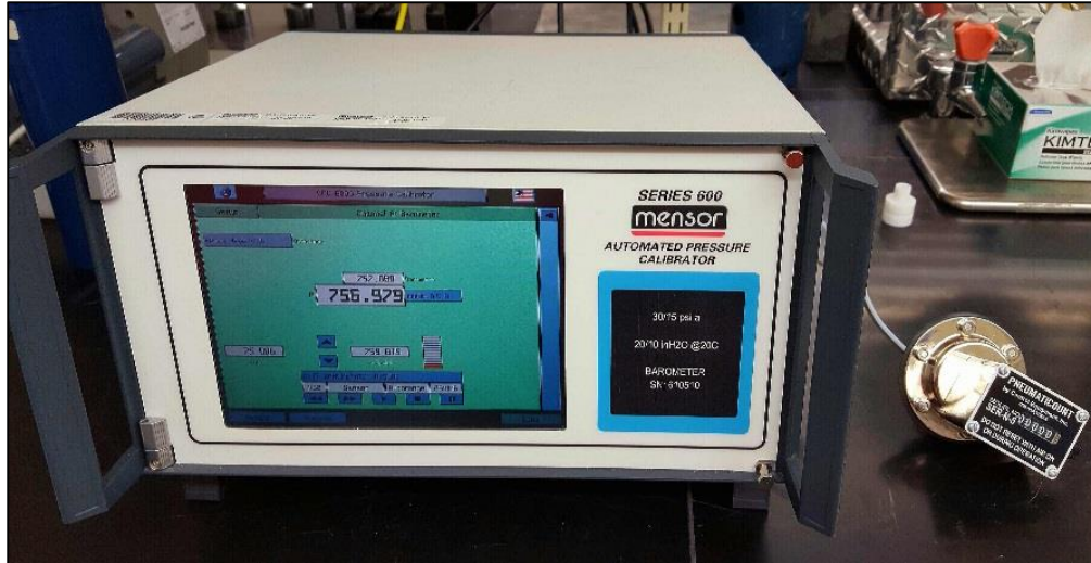
Figure 5-1. Mensor APC-600 with actuation counter attached.
