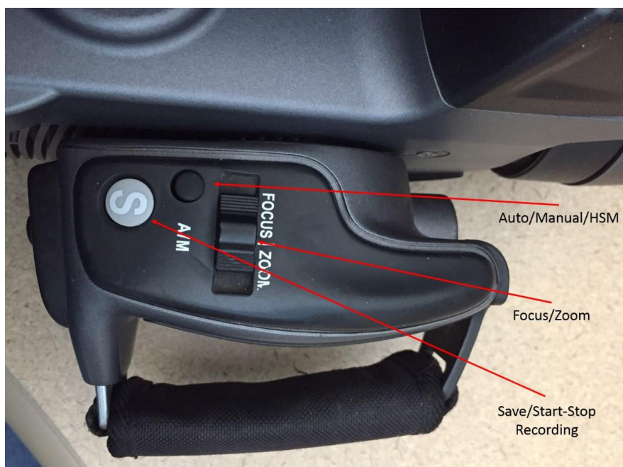
Figure 2. GF320 top of hand grip with Auto/Manual/HSM, Focus/Zoom, and Save/Start-Stop Recording buttons.
