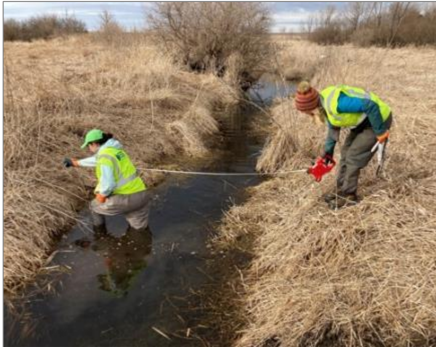
Figure 5. Measuring bankfull width. Image credit: James Treacy
