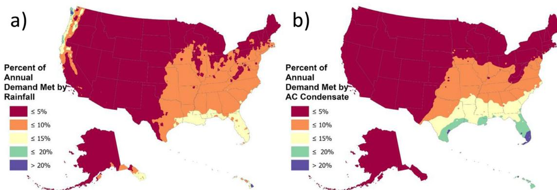
**Fig. 1.** Percent of annual non-potable demand met by RWH (a) and ACH (b) for a typical large building (Simulation Set 1, Table 1) having a total demand of 10.2 gpcd (38.6 lpcd).
