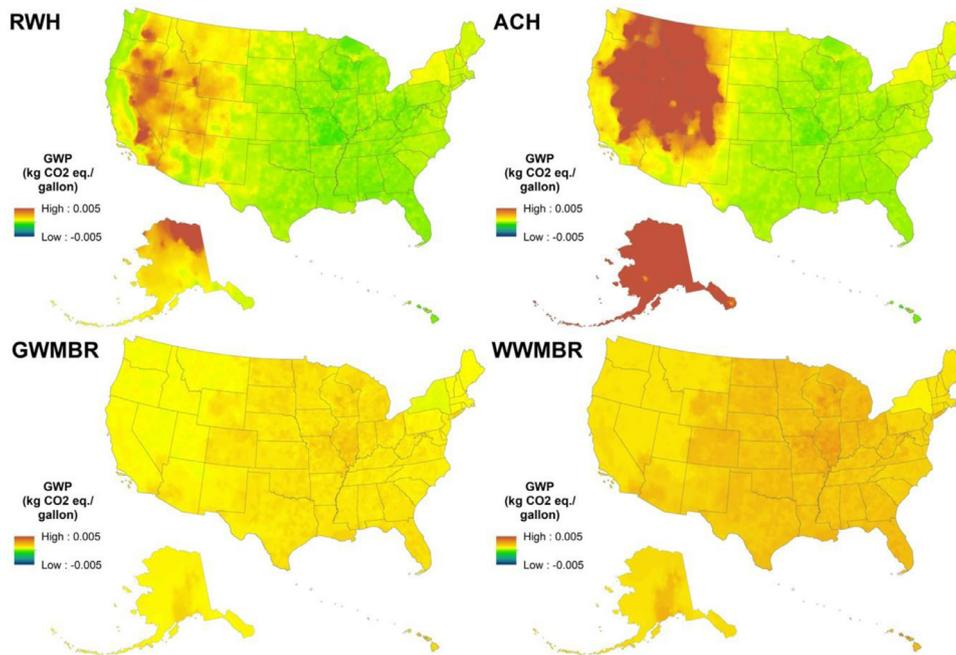
**Fig. 4.** Map of GWP impact of NPR system types for a large building (Simulation Set 1, Table 1).
