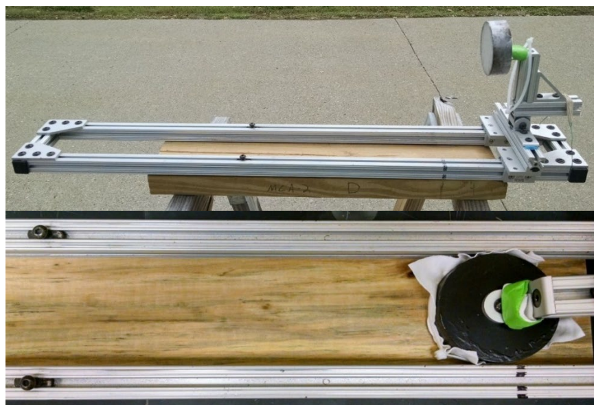
Figure S1: Wiping apparatus used in estimation of zinc and copper exposure through dermal contact. Apparatus was clapped to the board before sampling in the same location to ensure repeated sampling of the same surface over the prescribed time period. The aluminum disc (1.1 kg) was covered in a polyester fabric cloth and dragged over a distance of 50 cm. A wipe cycle constituted moving the weight back and forth 10 times, with the weight being rotated 90 degrees after the first 5 cycles.
