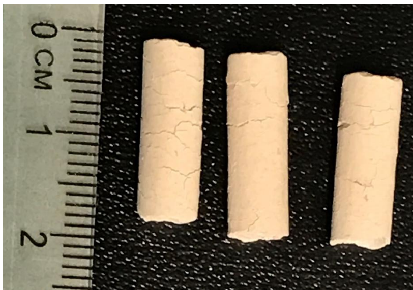
Figure 2 Pellets were synthesized with magnesium carbonate and cellulose for phosphate adsorption (photo by E. Martin).
