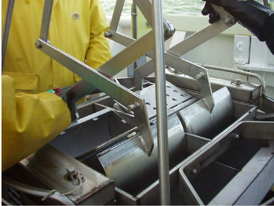
Figure 2.3.1. Close-up view of double Van Veen grab sampler used for bottom sampling.
