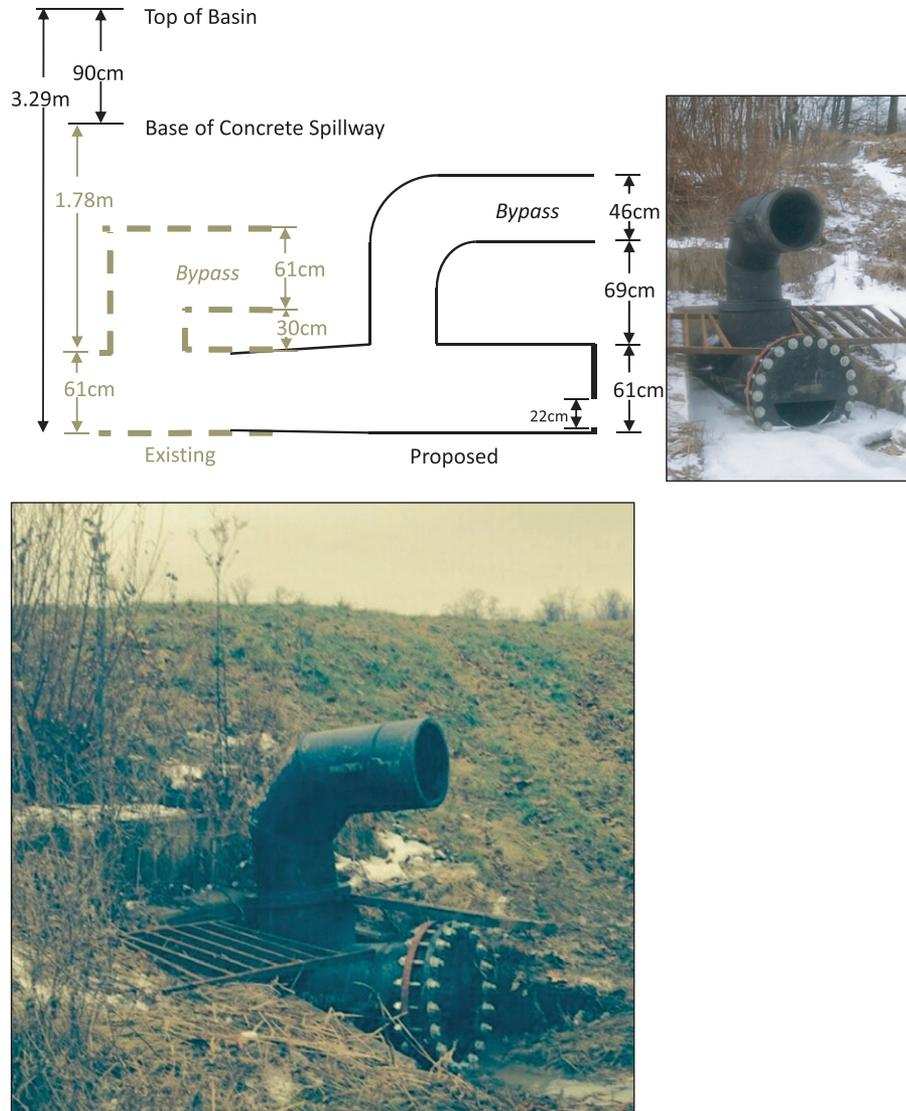
FIGURE 3. Design Schematic and Photos of Detain H<sub>2</sub>O Retrofit Device Pilot Installation.
