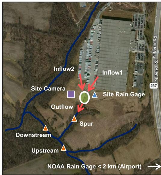
FIGURE 2. Pilot Installation Detention Basin (white and green oval) with Pipe Inflow and Outflow, Camera, Rain Gage, and Receiving Stream Monitoring Locations. Inflow from a swale entering from the east of the basin was ungaged.
